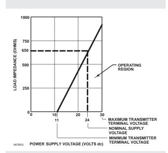
Figure 3. Transmitter Load Limitations
