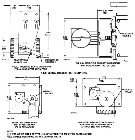
4200 SERIES TRANSMITTER (LONG STROKE) MOUNTING
