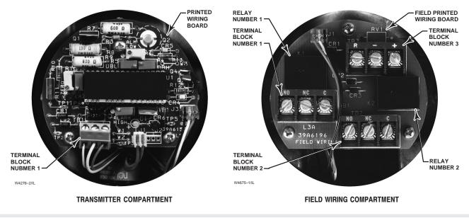
Figure 4. Type 4210 Transmitter Details
